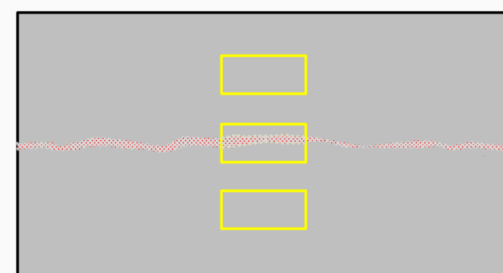
Fig.3: Schematic of a grain boundary showing rectangular boxes from where EDS or EELS measurements are performed using the spatial difference technique.
