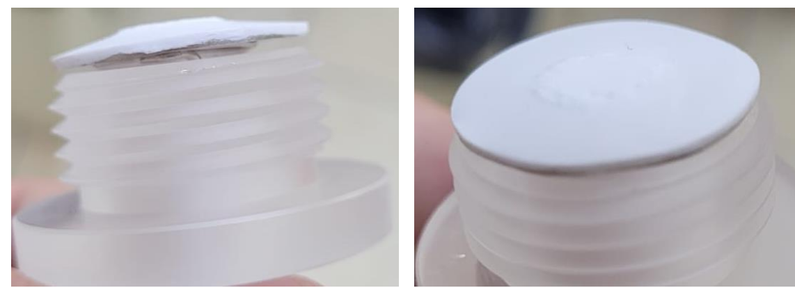
Figure 10: A noticeable deformation is present on the cathode after a series of annealing treatments for both 200 and 300 V/cm external fields. This deformation gradually increased with the use of the electrode and is accompanied by a mild dent in the inner face of the anode, where the samples are held.
