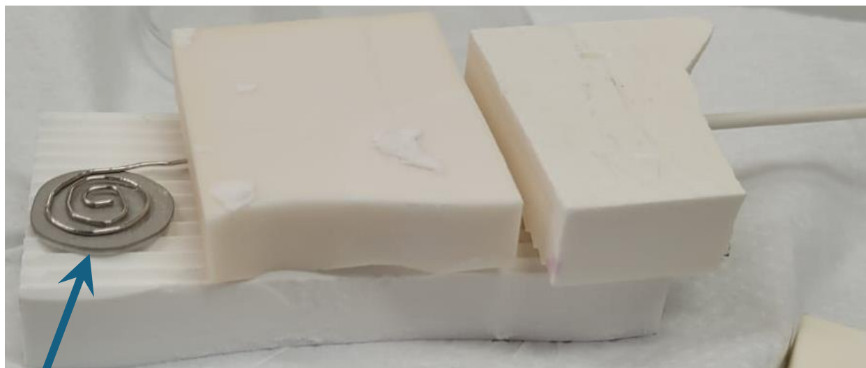
Figure 1: Disks were cut from sintered, undoped alumina, covered with Pt paste and thermally treated to form densified platinum layers on each electrode.
