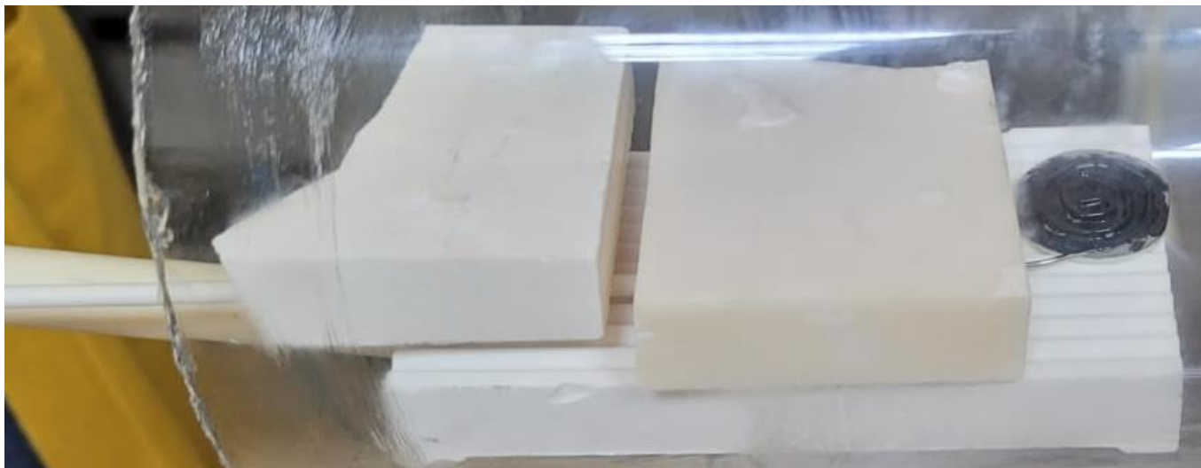
Figure 2: The platinum wire was placed against the already present platinum and coated with another layer of platinum paste to ensure constant contact during the annealing treatments.
