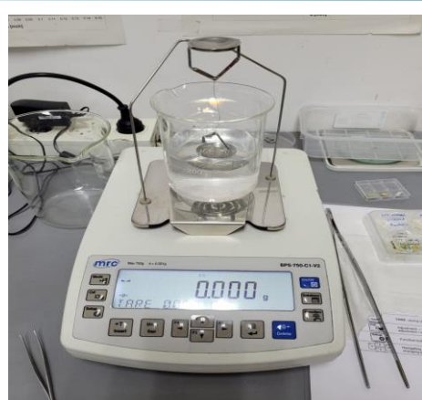
Figure 6: Density measurements were carried out via the Archimedes method prior to annealing. After the annealing treatments, samples were cut and polished for SEM observations to measure the grain size, relative to the distance from the electrodes.
