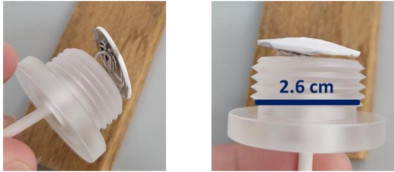
Figure 41: Photographs of the physical deformation observed in the positive electrode after using it for all of the aforementioned annealing treatments. A convex shape can be seen where the samples are normally in contact with the electrode. The outwards side of the electrode (coated with Pt paste) is curved inwards, and the layer of Pt paste is no longer uniform, particularly where the wire was brazed to the disk.
