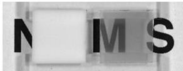
Figure 16: Alumina ceramics sintered by SPS at 1150°C at a heating rate of 100°C/min (left) and 8°C/min (right); reproduced from [46].
