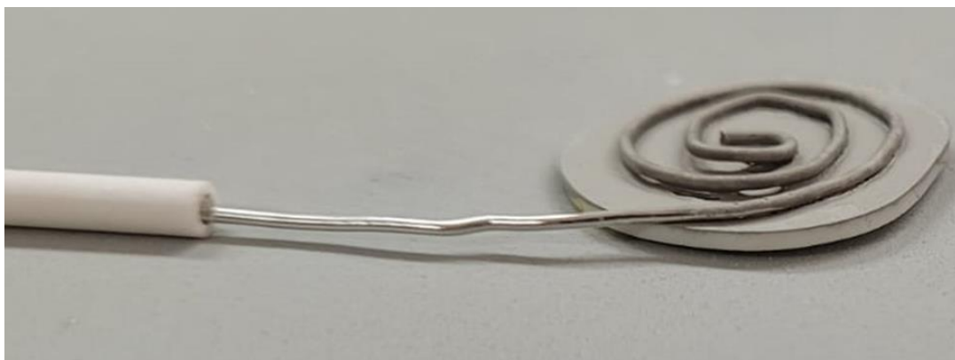
Figure 25: Photograph of Pt wire brazed to an alumina disk.
